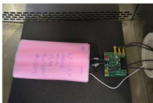
Sample Cell protected by an insulating film, a first tentative to get a uniform temperature on the cell.
