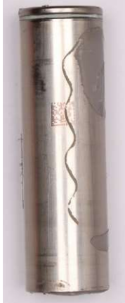
Figure 36 Panasonic 2170 cell taken from Tesla Model 3 battery for comparison tests on cell level
