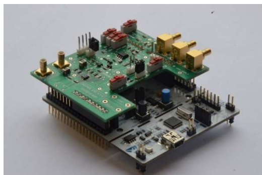
Figure 11 Non-working example of an embedded system performing the impedance estimation of a Li-ion cell. Here the algorithm computation is performed on a microcontroller.
